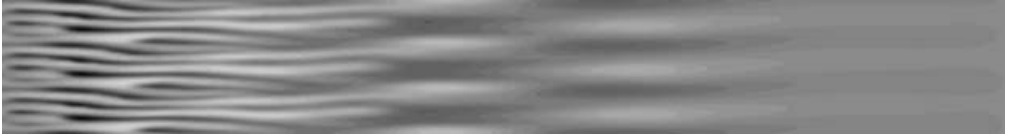
FIGURE 15. Instantaneous contours of streamwise velocity fluctuation ( -0.3 \leq u \leq 0.3 ). The plane is at y/\delta = 0.8 . The spanwise coordinate is enlarged by a factor of 3. Inlet modes: \omega = 0.032 , k_y = \pi , k_z = 4.7 , \Theta = 32.5 and \omega = 0.064 , k_y = 4\pi/3 , k_z = 3.5 , \Theta = 10.1 .
