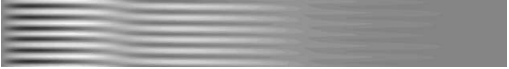
FIGURE 12. Instantaneous contours of streamwise velocity fluctuation ( -0.3 \leq u \leq 0.3 ) evaluated at y/\delta_0 = 0.58 . The streamwise extent shown is 0.4 \times 10^5 \leq R_x \leq 2.4 \times 10^5 . The spanwise coordinate 0 \leq z \leq 8 is enlarged by a factor of 3. Inlet mode: \omega = 0.032 , k_y = \pi , k_z = 4.7 , \Theta = 32.5 .
